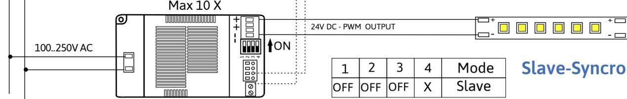
Syncro Line: use data BUS cable, keep away from high voltage line to avoid interferences.
